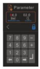
Touch the parameter or by pressing "♥" "♥" select the number that needs to be changed, it will light red, or by pressing the numbers adjust it. To save press "←"
