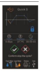
If the cycle is manually interrupted after it reaches the drying phase, the items inside the sterilizer may be considered sterile.
