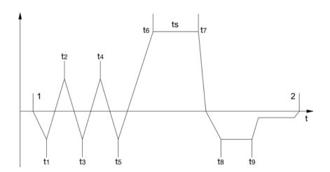
Program: WRAPPED Temperature: 134C Pressure: 206.0 kPa Drying Time: 08Min Holding Time: 4.0Min
