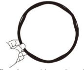
Press the remaining sections of the seal.
